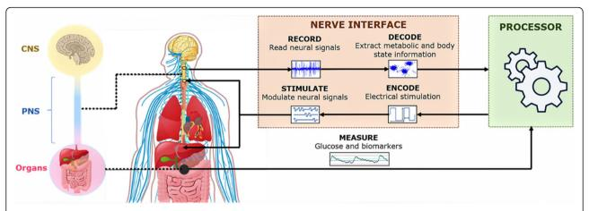
**Fig. 1** A depiction of future closed-loop neuromodulation systems for diabetes management. Metabolic biomarkers and neurophysiological recordings from a variety of peripheral nerves can be used to automatically control the stimulation dosage to be delivered back to the peripheral nervous system or directly to the organs to modulate their function
