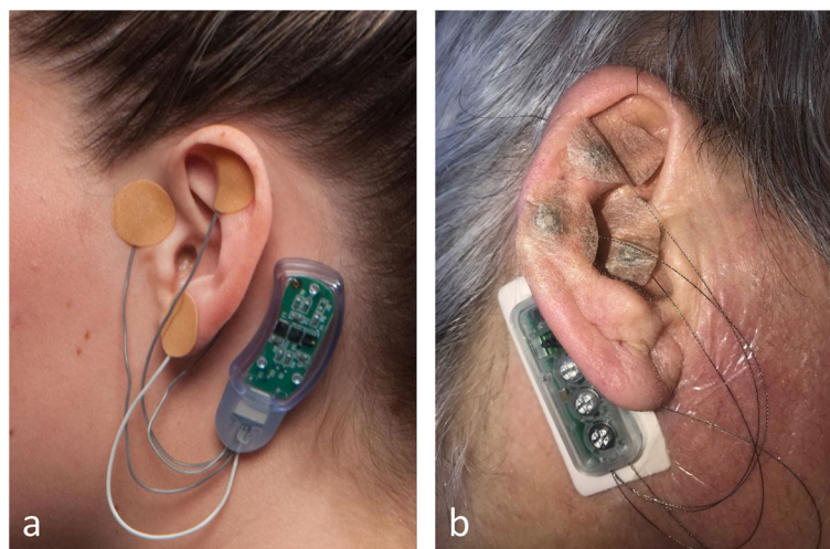
Fig. 1 a The NSS-2 Bridge device placed on the ear. The body of the device is placed behind the ear. The stimulating electrodes are connected via wires and placed at key points on the ear. Each electrode contains a short penetrating needle which is used to provide percutaneous electrical stimulation. Source: Forbes.com : (source) b The DyAnsys Drug Relief stimulator placed on the ear. The device is similar in construction to the NSS-2 Bridge device which served as the predicate for its approval. (source)
