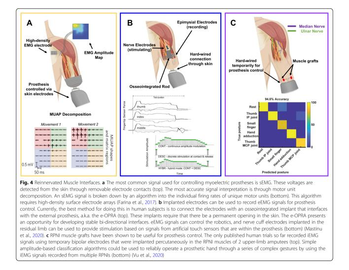
Compensation) (Farina et al., 2014). The algorithm's job is to "decompose" the raw sEMG signal to identify motor unit spike waveforms and their firing rates (Fig. 4a, bottom). Decomposing an sEMG signal is like listening to the recording of a symphony orchestra and then determining the exact musical notes being played by each instrument.
